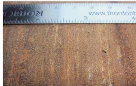
Material plating on the shaft liner
